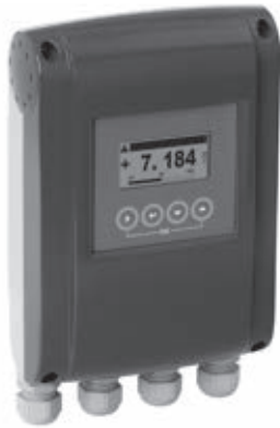
(signal converter in wall-mounted aluminium housing)
